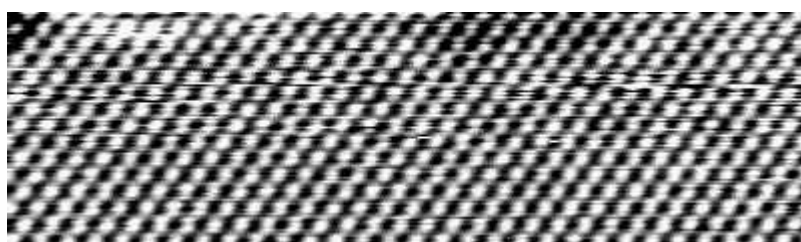
Figure 7.2: Atomically resolved STM image of the 2D Ho silicide surface. Imaged acquired at a bias voltage of 2V, tunnelling current 2nA. \sim 10 nm \times \sim 3 nm.
